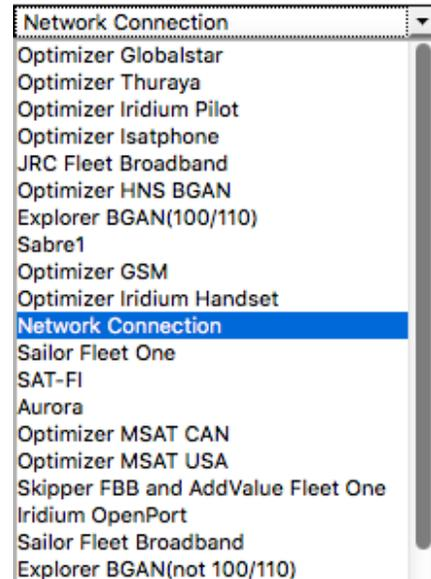
Unmanaged connections are intended for satellite terminals configured to be online all the time. Select “Network Connection” from the drop down list; and, configure the satellite terminal to automatically connect to the Internet on network traffic. This unmanaged configuration typically results in lower airtime use since the number of connections incurring minimum billing increments is reduced.
