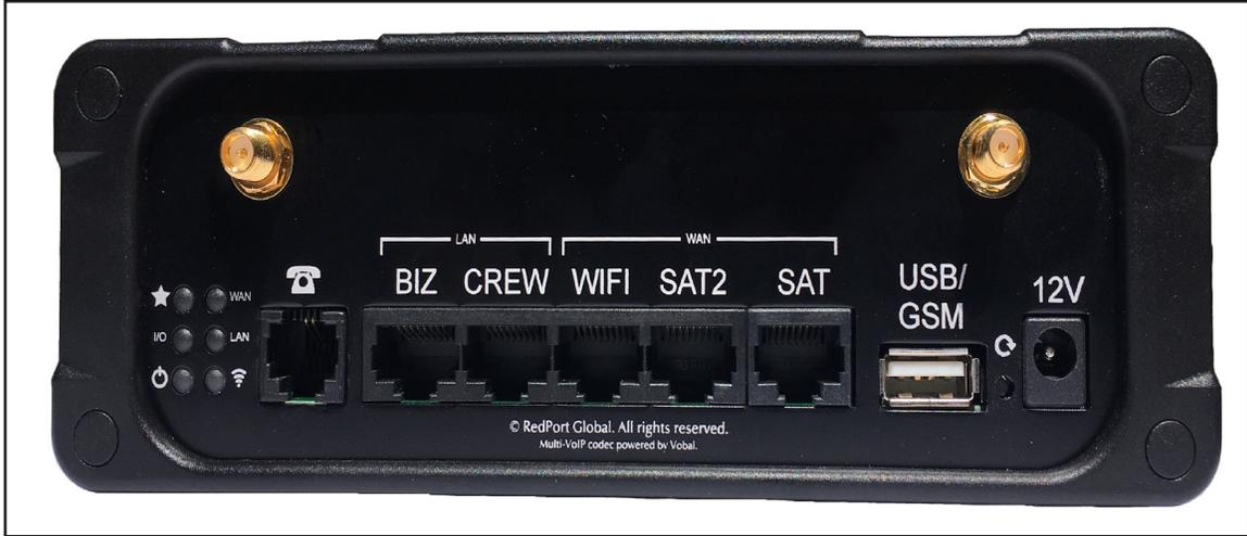
Connect the NMEA device to the USB port on the rear of the Optimizer CrewComm with an appropriate USB to Serial Adapter.
