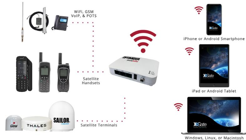
The RedPort Optimizer is a satellite Wi-Fi router that combines a powerful satellite data router with voice capabilities, including a full PBX. It is more than just a voice device. It gives you everything you need to create a local voice and data network with your satellite device. Built-in firewall protects your satellite data stream from unwanted traffic and prevents high airtime bills.
