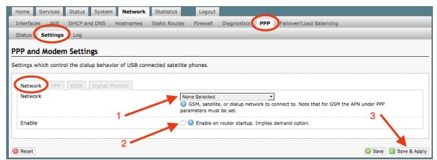
Use the following to configure the PPP interface for use with a GSM modem.
