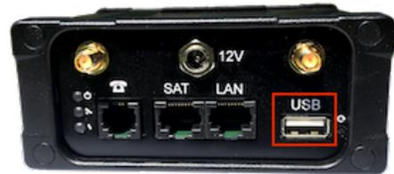
Connect the NMEA device to the USB port on the rear of the Optimizer with an appropriate USB to Serial Adapter.
